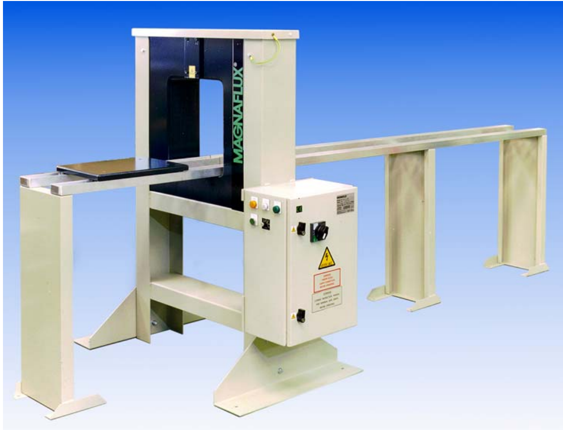
SB Units as illustrated offer up to 12,000 ampere turns as an option to the standard 8,000 ampere turns
